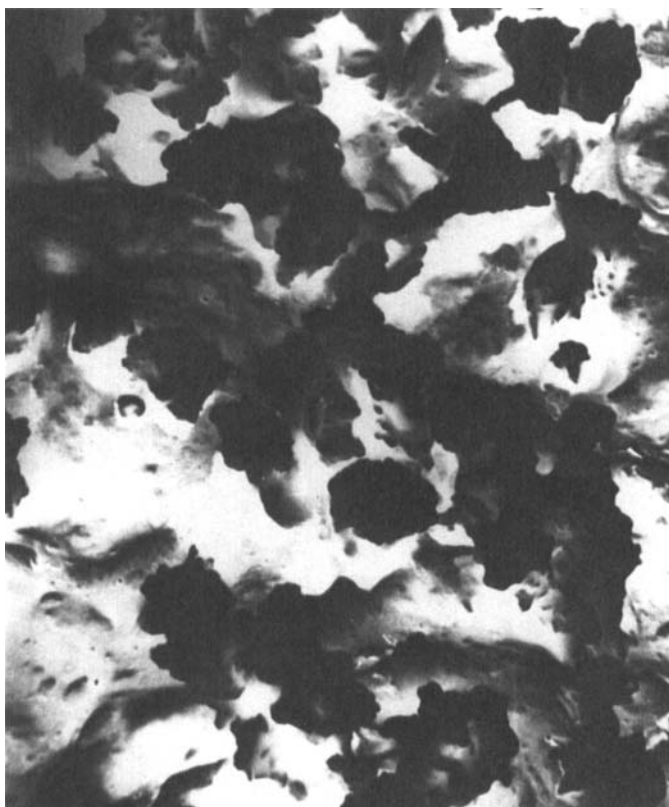
FIG. 5. SEM photograph (1 000 \times ) of chlorophosphazene-Ultrazine NAS reaction product modified by diethylamine (No. 8).
