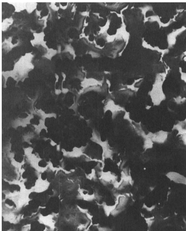
FIG. 4. SEM photograph (1 000 \times ) of chlorophosphazene-Ultrazine NAS reaction product (No. 6).
